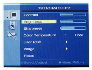
b. Press " $_{\triangle}$ " or " $_{\nabla}$ " to increase or decrease the brightness of the display. Press "1" to confirm the adjustment and back to OSD main menu.
